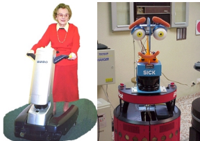
Figure 2. Guido the smart walker (left), and Urbano the interactive tour guide robot (right)
